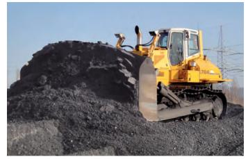
Spreading coal on the tip
