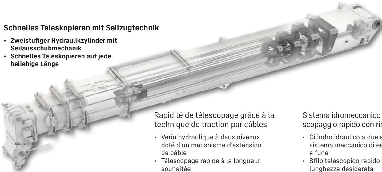
Telescoping with rope pulling technology
