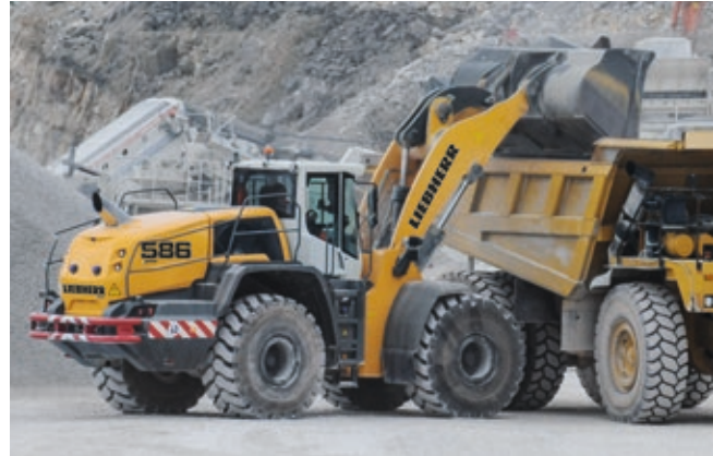
The L 586 XPower® wheel loaders have been specified with longer lift arms for loading the quarry trucks.
