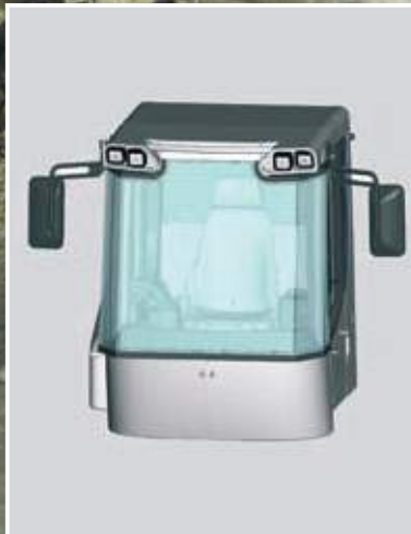
Cab with laminated safety glass
