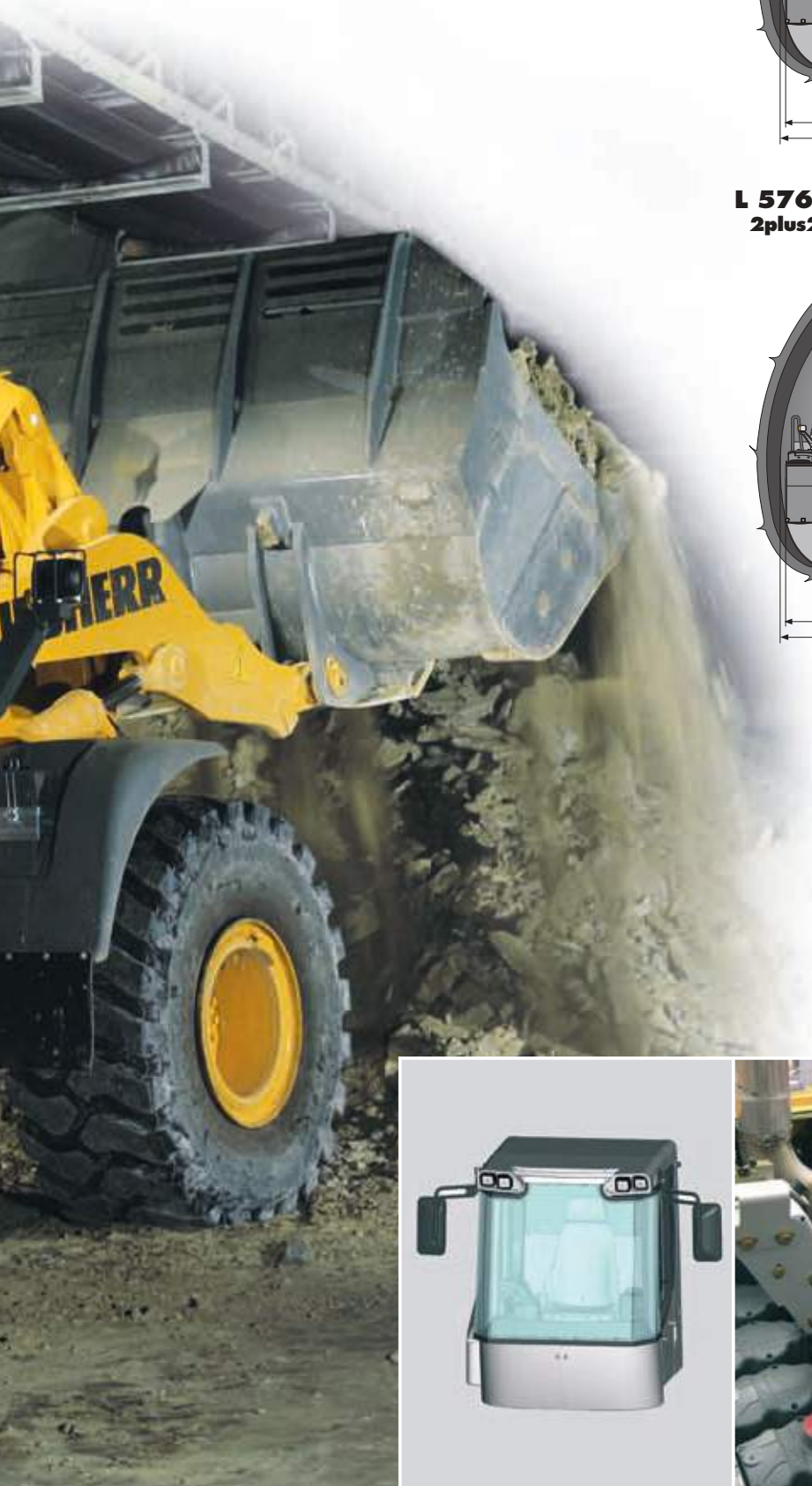
Cab with laminated safety glass
