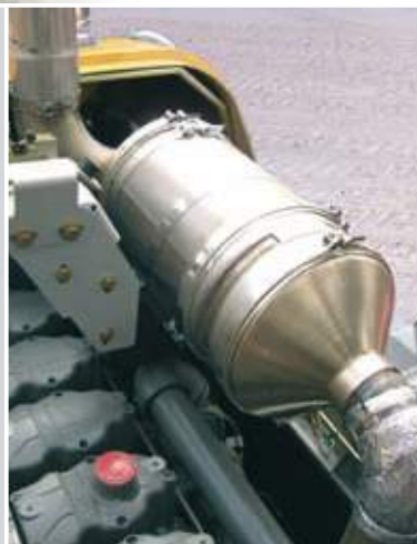
Diesel particle filter beneath cladding
