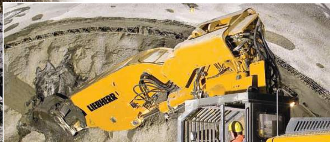
Protection for boom and hydraulic cylinders
